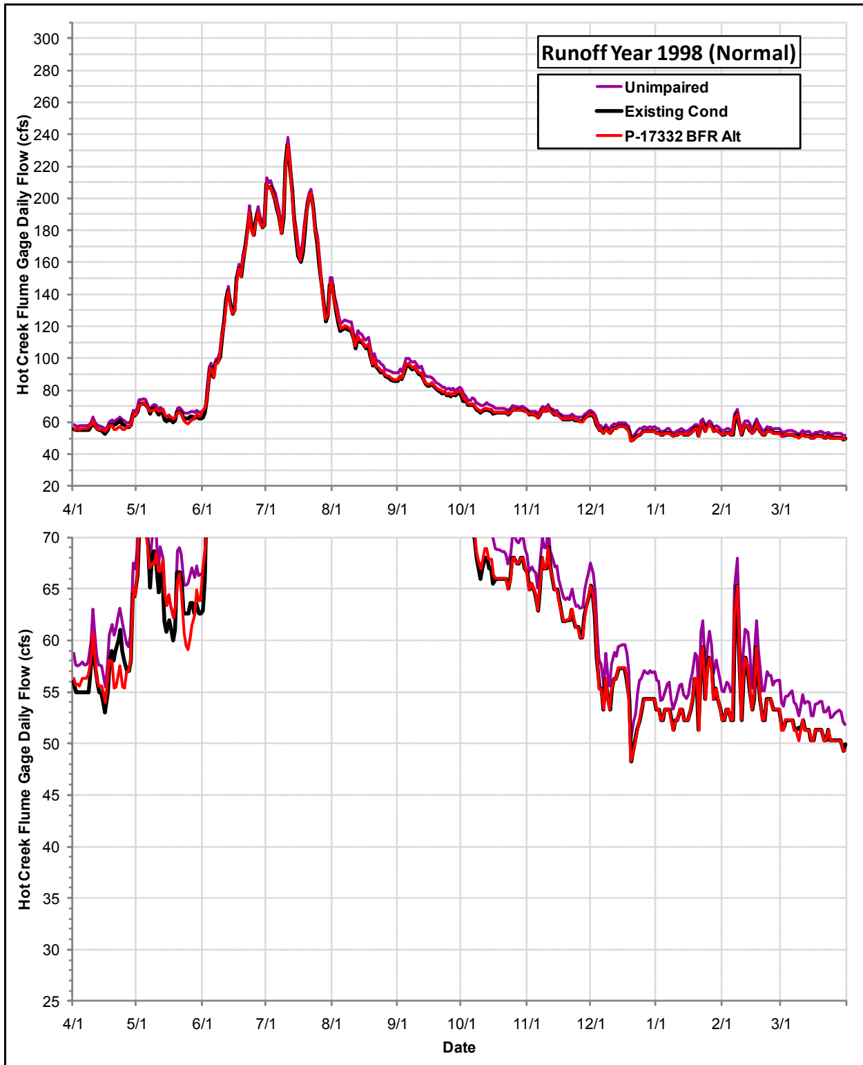
Daily Flows (cfs) at the USGS Hot Creek Flume Gage under the Permit 17332 Bypass Flow Requirements Alternative, the Existing Condition and the Index of Unimpaired Conditions during Runoff Year 1998
